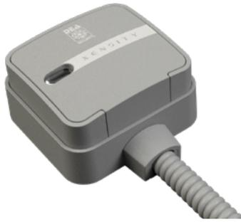
Microprocessor analysis board for SN-XS-GR sensors. It processes the analog signals coming from SN-XS-GR sensor and sends the alarm signals (if any) to the Controller board through XENSITY Bus. BR-XS-GR can discriminate between cut (continuous vibrations), shock (weak impacts) and breakthrough (strong impacts); it also allows filtering nuisance alarms due to thermal expansion of the metal structure.
