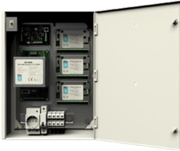
Polyester cabinets, factory-assembled according to the project specifications. They provide inputs and outputs on DIN rail terminal board and integrate a shock detector to signal forcing and breaking-through.
