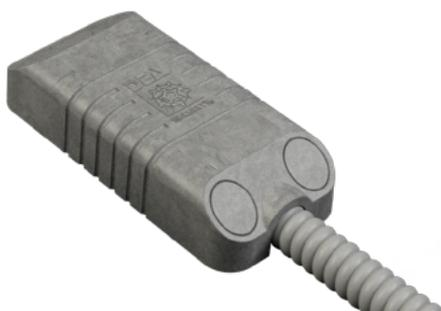
Piezoceramic passive sensor which protects metal burglar bars against shock, cut and breakthrough. Designed for outdoor use, the sensor is protected by a reinforced polyamide housing and the connection cable is wrapped with flexible metal conduit.
