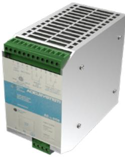
Stabilized switching power supply unit (mark Adelsystem) with 24 Vdc output voltage and 3 A max output current. It provides two relay outputs: one for mains or backup and one for low or discharged battery.
