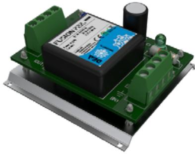
Electronic voltage regulator (booster) to be coupled with the BR-FSP2PLT-CTRL control board. Its function is to step up voltage from its input (12V) to its output (24V) ensuring the maximum sensor bus stability at full load.
