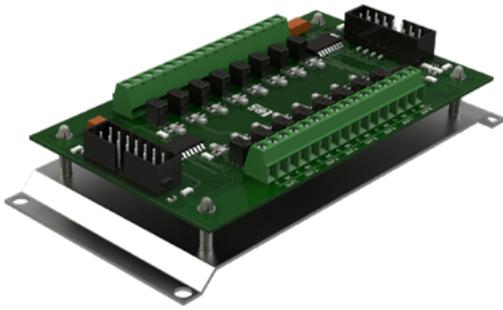
16-relay expansion board to make the alarm signals available through C/NC contacts.
