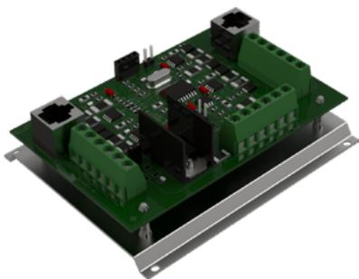
Interconnection board which connects DEA Security processing boards to DEA NET. This board amplifies and regenerates the signals over DEA NET, making it possible to cover long distances.
