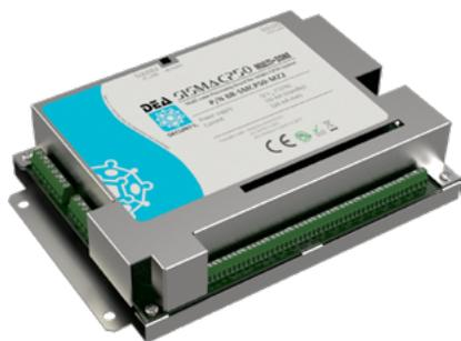
Electronic processing board which manages two SISMA CP 50 sensor-strings. It amplifies, digitizes and analyses the signals coming from the sensors, discriminating the typical signals of an intrusion event from the ones generated by environmental nuisances. The board is equipped with Ethernet interface and IP native support.
