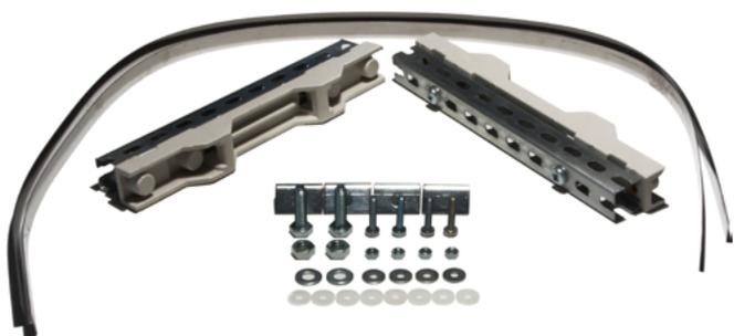
Kit to mount the AP-1C, AP-2C, AP-3C and AP-4C cabinets to the poles. It includes two metal straps 125 cm long, two brackets and the relevant mounting hardware.
