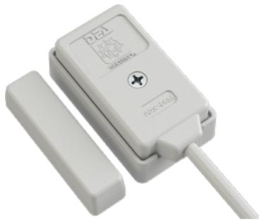
Piezodynamic shock detector to protect windows and doors against shocks, opening and breakthrough attempts. Door, window or skylight frame mounted, its high detection capability enables it to protect the whole structure, including glasses.
