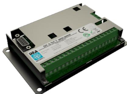
Interface board which allows sending over DEA NET the signals generated by third-party equipment. It has 4 triple balanced analog inputs, 4 digital inputs and 2 relay outputs for the activation of third party devices.
