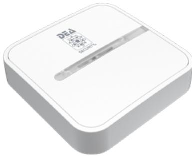
Dual-tech seismic detector for the protection of walls and armoured structures against breaking, breaking through and drilling events. It can be installed at any inclination and orientation on different types of walls, including masonry, tuff, reinforced concrete and metal (e.g. vaults, safes and security cabinets). It employs tamper devices to signal sensor removal, thermal sabotage and case opening attempts.
