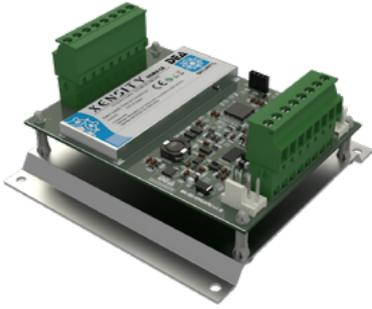
Interface board for one SISMA CA/CA PF sensor-module which amplifies the signals coming from the sensor-module and transmit them to BR-XS-CTRL32/64 board by means of XENSITY bus.
