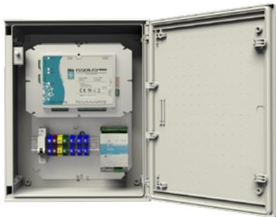
The control unit manages up to 300 detectors on 2 communication buses for maximum 1.500 metres of perimeter if the spacing between the sensors is 5 metres and 900 metres of perimeter if the spacing is 3 metres. Besides enabling the configuration of the detectors by means of a service software, the control unit automatically recognizes and sorts the field detectors and raises the alarm signals.
