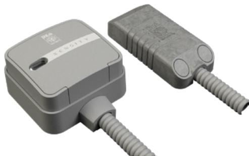
Module for the protection of metal burglar bars against cut, shock and breaking through. It is composed of SN-XS-GR piezoceramic sensor equipped with cable protected by flexible metal tube and of BR-XS-GR addressable peripheral analysis board. The latter manages two triple balancing lines for the connection to third-party devices equipped with C/NC contact.
