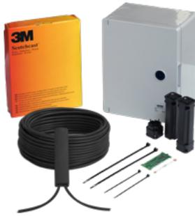
Module for the protection of a rigid fence up to 50 metres long. It is composed of a prewired sensor-string of 20 sensors for the protection of fence panels with 2.5 metres width, a preassembled Analysis Unit, a 25-metre hank of cable and a wiring kit.
