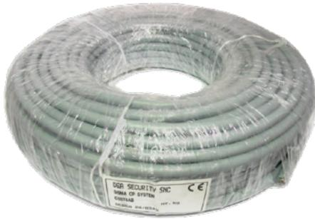
Tinned copper six-wire shielded cable with rodent-proof armour. It is used to connect LN-SMCP50 sensor-string and SN-SMCP50 sensor prewired in a string to BR-SMCP50-Z1 or BR-SMCP50-Z2 processing board.
