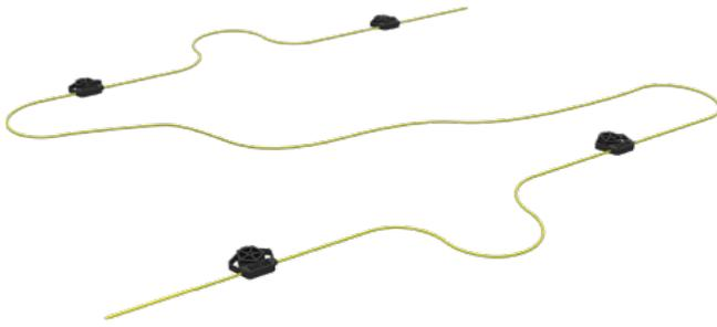
Prewired sensor-module for the protection of raised floors with a surface between 6 and 24 square metres. The sensor-module is composed of 4, 6, 8, 12 or 16 pressure sensors and is provided with prewired termination and 5-metre initial cable.
