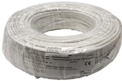
2-conductor shielded cable for the connection of A03 PRO sensors to BR-A03P-Z4 processing board. Compliant with CEI-UNEL 36762, it is suitable for fixed installations in buildings and other civil engineering works subject to reaction-to-fire requirements.
