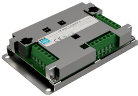
High-insulation version of SC-DN-HTRPT board to be used in environments highly disturbed by electromagnetic inductions. The three ports on the board are galvanically isolated (with isolation voltage up to 2500 VRMS), guaranteeing a high immunity to possible environmental disturbances along the communication line.
