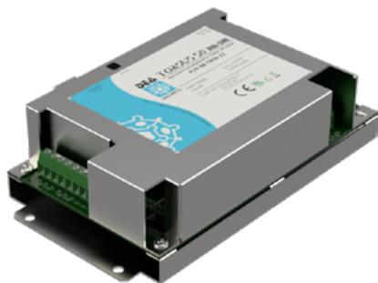
Electronic processing board which manages two TORSUS 50 sensorstrings. It amplifies, digitizes and analyzes the signals coming from the sensor-strings, discriminating the typical signals of an intrusion from those generated by environmental nuisances. The board is equipped with Ethernet interface and IP Native support.
