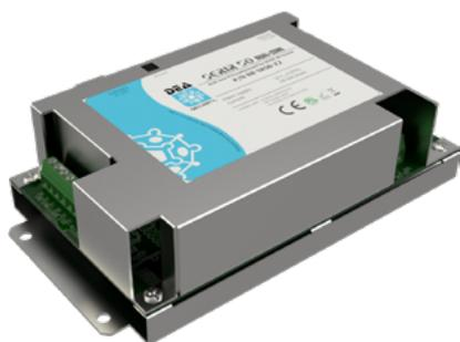
Electronic processing board which manages four SERIR 50 sensor-strings.
