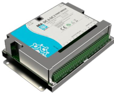
The electronic controller board for Ethernet network manages up to 16 DEA Security electronic analysis boards. It checks the operating status of each single board and collects the related signals, saving the latter to an internal memory and make them available through dry contacts, over DEA NET proprietary network or over IP network. The service software allows monitoring and configuring, locally or remotely, all the analysis boards and the relais expansion boards (if any) connected.
