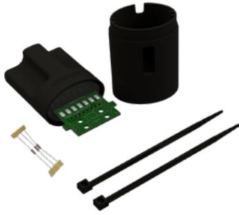
Peripheral module containing an electronic interface board for the management of a resistive balanced input. It can be connected everywhere along the sensor-string and allows you to integrate into the system signals coming from third-party devices such as magnetic contacts. The printed circuit board is protected by a polyamide housing which provides a very high resistance to UV rays and scratch.
