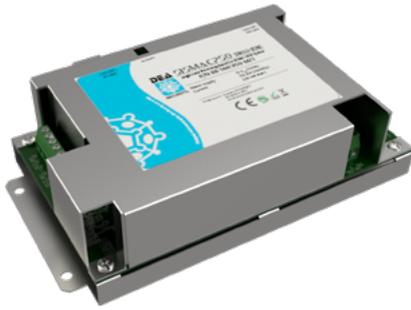
Electronic processing board which manages one SISMA CP 50 sensorstring. It amplifies, digitizes and analyzes the signals coming from the sensors, discriminating the typical signals of an intrusion from those generated by environmental nuisances. The board is equipped with Ethernet interface and IP Native support.
