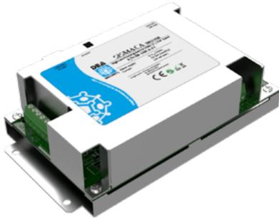
Microprocessor electronic board which manages one SISMA CA or SISMA CA PF sensor-module. This board amplifies, digitizes and analyses the signals coming from the sensor-modules, discriminating the typical signals of an intrusion attempt from the ones generated by environmental nuisances. The board is equipped with Ethernet interface and IP Native support.
