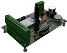
Microprocessor electronic board which manages one TORSUS 50 sensor-string. This board amplifies, digitizes and analyses the signals coming from the sensor-string, discriminating the typical signals of an intrusion from the ones generated by environmental nuisances.
