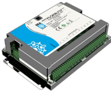
Electronic control board which powers and manages up to 100 FUSION P2P sensors on a single communication bus. It performs several functions among which the automatic acquisition and sorting of the sensors, the processing of the alarm signals and the native support to the centralization and remote management of the system over IP networks or DEA NET proprietary network.
