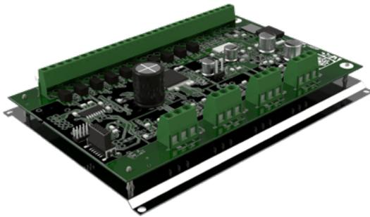
Multi-zone digital processing board to manage all SERIE A03 PRO sensor models. It processes the signals coming from the detectors and generates alarm states. The service app displays the alarms differentiating them by type of attack: shock (low shocks), breakthrough (gross attacks), drilling (continuous shocks).
